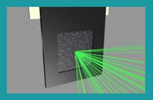
Scheme of the experimental set-up: The chip loaded with nanocrystals is scanned by the fine X-ray beam (green) pore by pore. Ideally, each crystal produces a distinctive diffraction pattern. Photot: Philip Roedig, DESY
